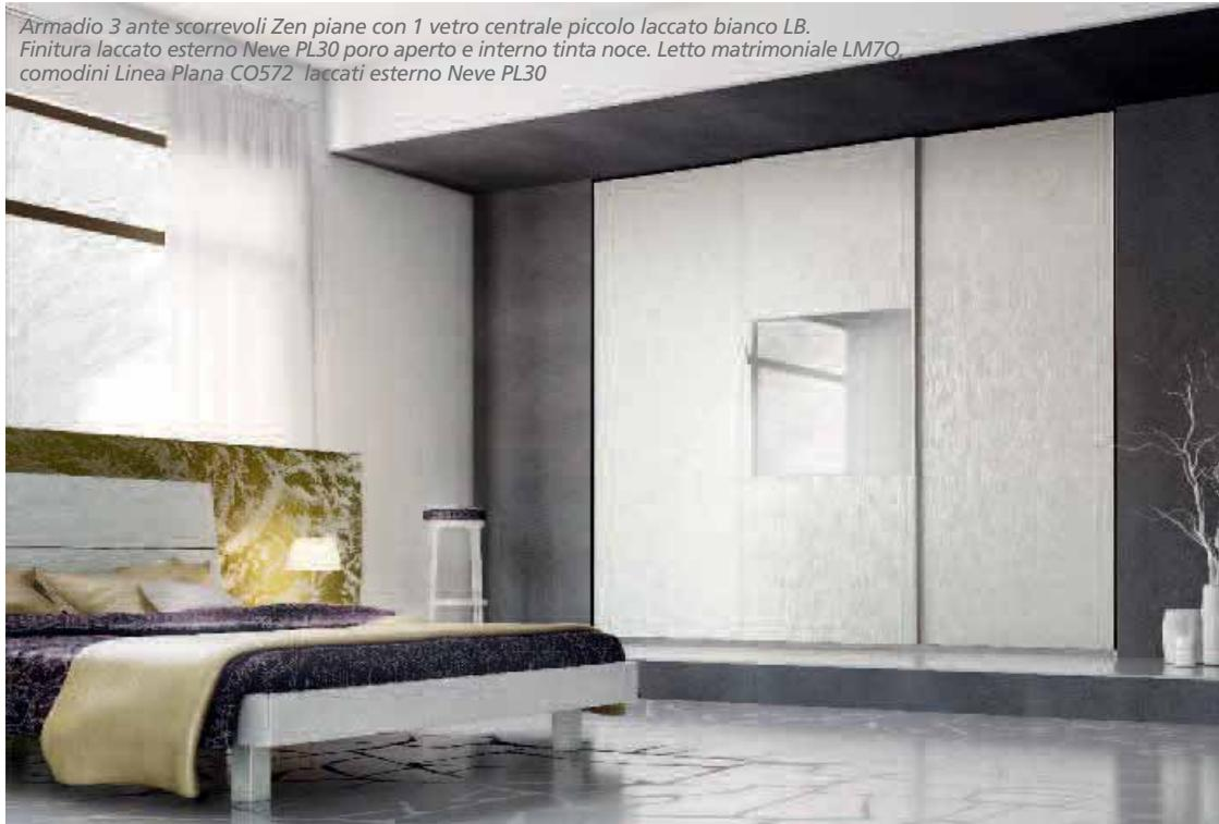
The sliding doors Zen project shows great versatility of dimensions and is available in height cm.262, cm.296 and can also be cut to measure. The width are cm.205, 306, 407, 456.5, and so on, passing through basis doors (w.cm.104) and XL doors (w.cm.154.5, in 3 pieces). Depths cm.57.6- 38.4- 24.1 plus doors (cm.8)
